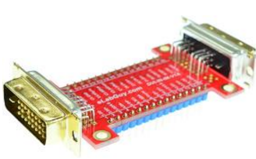
Figure 3: DVI-DM-DSM-V1A with headers
